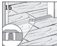
An expansion gap T-strip is required when length of planks measures 40' max and when width of planks measures 25' max. Transition strips should be placed in all doorways directly under the door when the door is closed.
