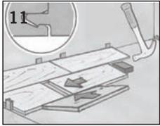
Use a 4"- 6" piece to hold the tongue and the groove on the same plane, limit end joint damage and ensure planks engage square. Tap end joints with multiple light taps, striking the tapping block evenly until end joints close.
