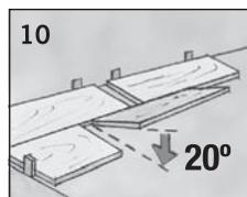
10 Lock in panel lengthwise. Allow 12" minimum end-joint stagger row to row.
