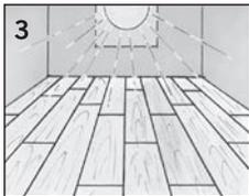
3 Install parallel to main light source; if no exterior light source, install parallel to longest wall.
