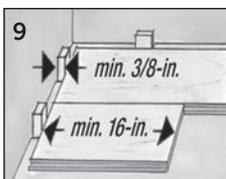
9 Observe 3/8" clearances for expansion and 16" minimum for smallest usable piece.
