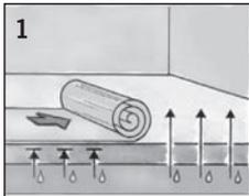
1 Install vapor barrier if subfloor is cement (6 mil polyethylene film).
