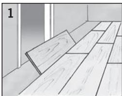
Some long edge joints cannot be installed using a 20° angle.
