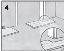
4 If possible, start to lay panels under the door jam and finish installing planks on a wall without a door jam. See Working with Limited Clearance section.
