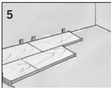
5 Start placing panels so that tongue sides face the wall.
