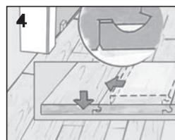
Slide panel into space horizontally and slot into profile. Use these modified planks under doorframes, radiators, cabinet fronts, etc. Use the pull bar to slide the planks where needed.
