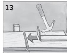
Fit the last panel in the row using a pull bar.
