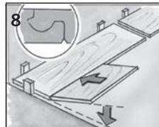
8 Rock and lock in half-length panel with rotating motion. Install first and second row at the same time. This will help ensure end joints are perfectly square. Planks forced down without properly engaging the tongue into the groove can result in damage.
