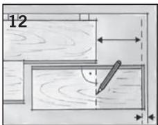
To measure and cut last piece in a row, rotate offcut section 180°, mark accordingly, cut, rotate back 180° and slot into space.
