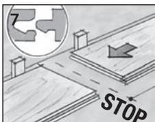
7 Lay panels close together on floor.
