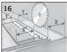
Cut the row along the wall to account for the unevenness of the wall while leaving 3/8" expansion room (2.5" minimum plank width).
