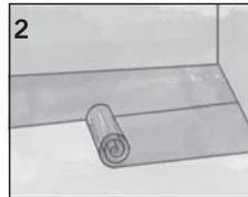
2 Always use an underlayment padding above the vapor barrier and below the laminate flooring planks. If pad is pre-attached, no additional underlayment should be used.
