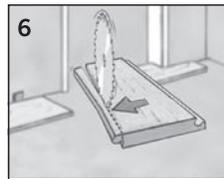
6 Remove the tongue on the panels that face the walls to allow room for spacers and prevent problems from spills.
