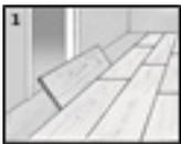
Some long edge joints cannot be installed using a 20° angle. Use good quality wood glue to make the connection.
