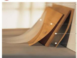
The top layer, known as the wear layer, protects against staining, fading and wearing. It is made from translucent paper (wood fibre), impregnated with moisture repelling resin and abrasion resistant aluminum oxide, which is roughly as hard as diamonds.
