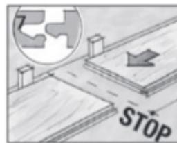
Lay panels close together on floor
